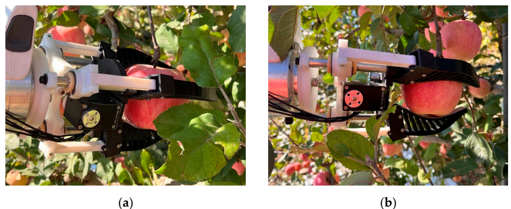
Figure 24. Gripper attitude with force feedback on and off: (a) force feedback on; (b) force feedback off.
