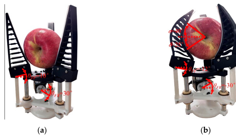
Figure 20. Contact model of soft gripper: (a) initial contact; (b) full contact.
