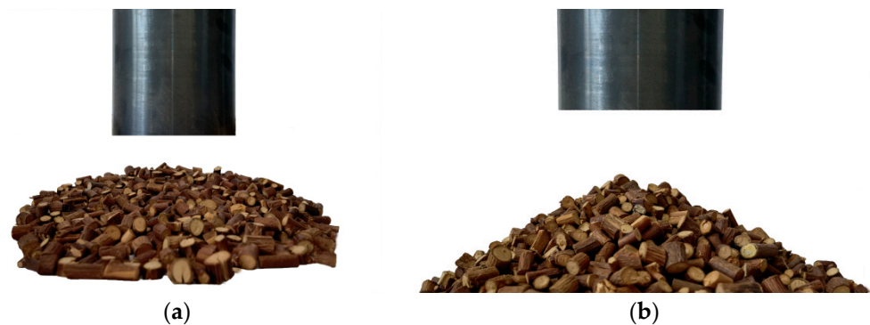
Figure 5. Physical test of repose angle: (a) the circular chassis substrate; (b) stacking test results.
