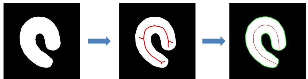
Figure 6. Rendering of the mesh pruning algorithm.
