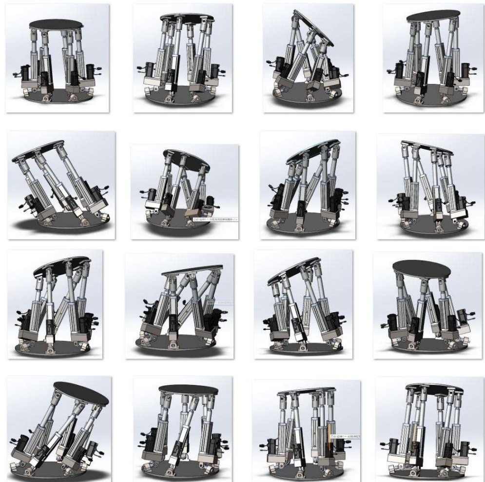
Figure 7. Interference verification of 16 extreme positions and postures of lifting platform.
