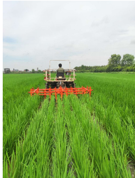
Figure 9. Weeding effect of reciprocating inter-row paddy weeding machine for strip-seeded rice.
