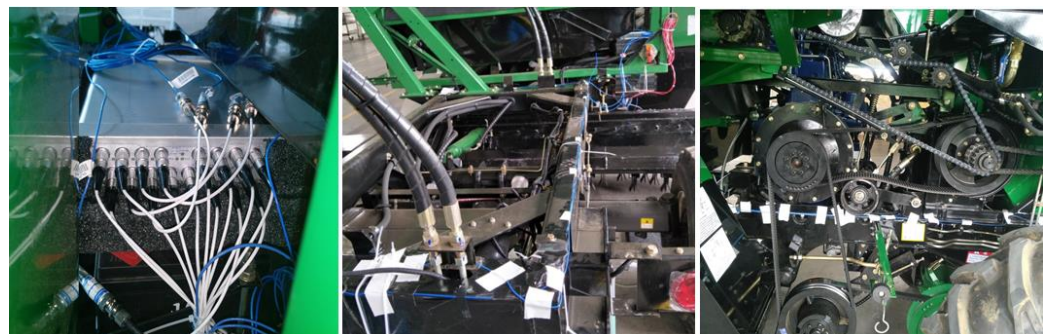
Figure 2. Operating modal test of the harvester frame.
