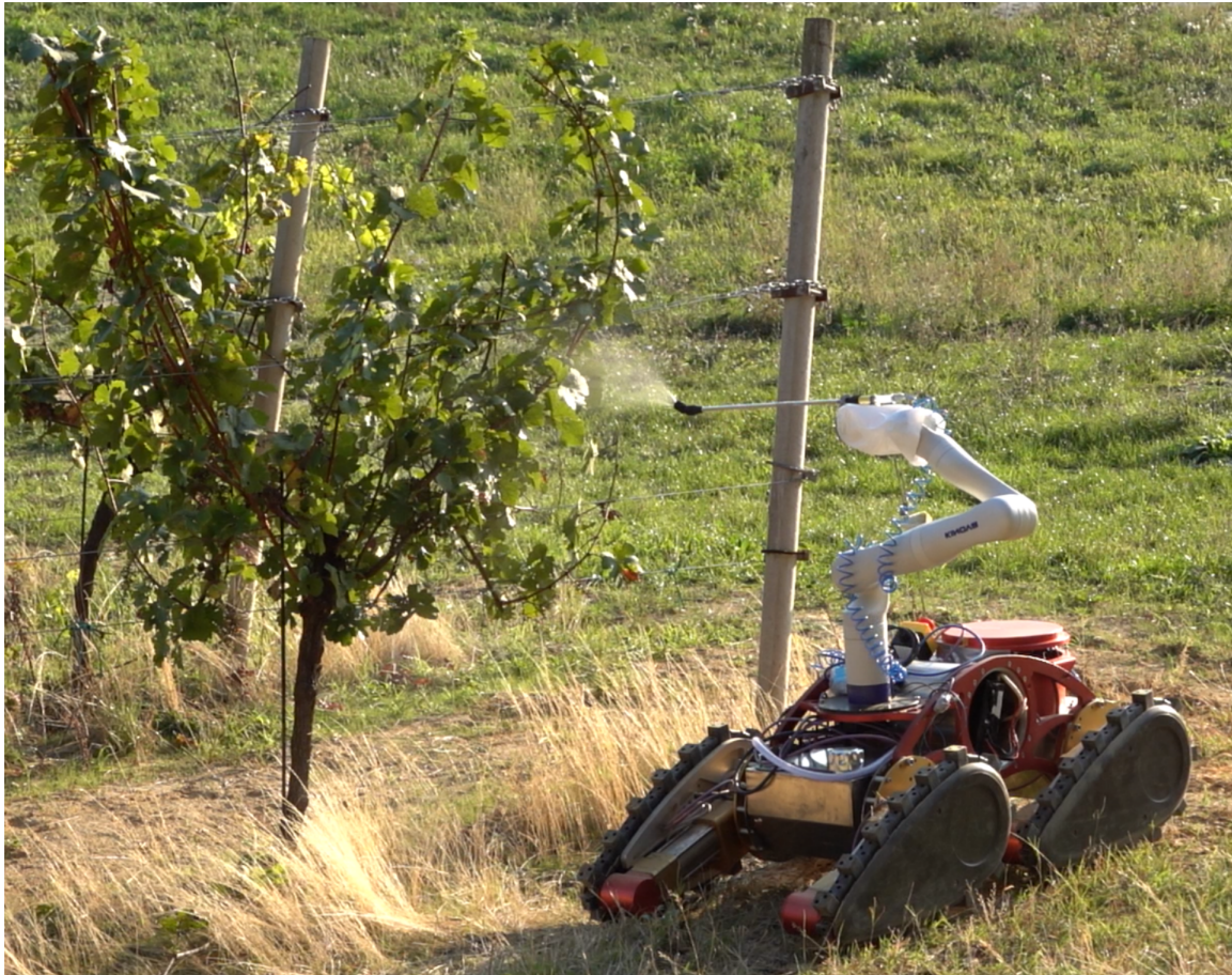
Figure 8. Mobile manipulator performing a spraying experiment in a vineyard.
