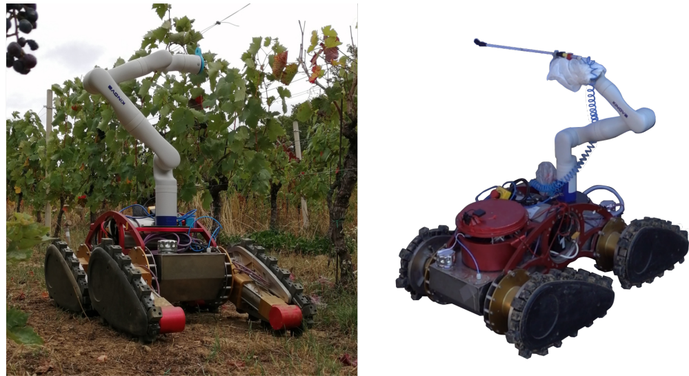
Figure 1. Mobile manipulator developed for the HEKTOR project, with an emphasis on manipulation ability and maneuverability in steep terrain.
