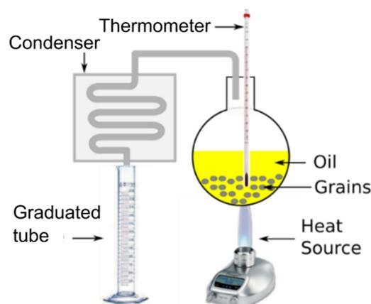
**Figure 3.** Diagram of the method of determination of humidity by distillation.
