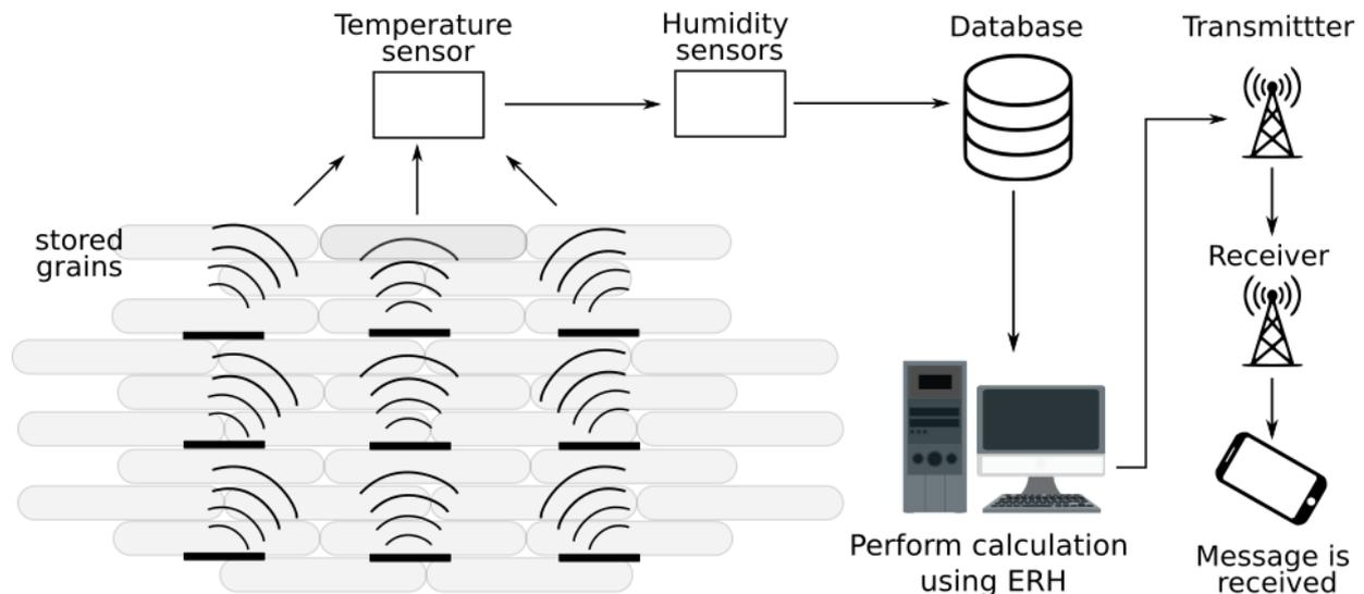
**Figure 16.** Schematic of system to sense moisture grain with ERH calculus.
