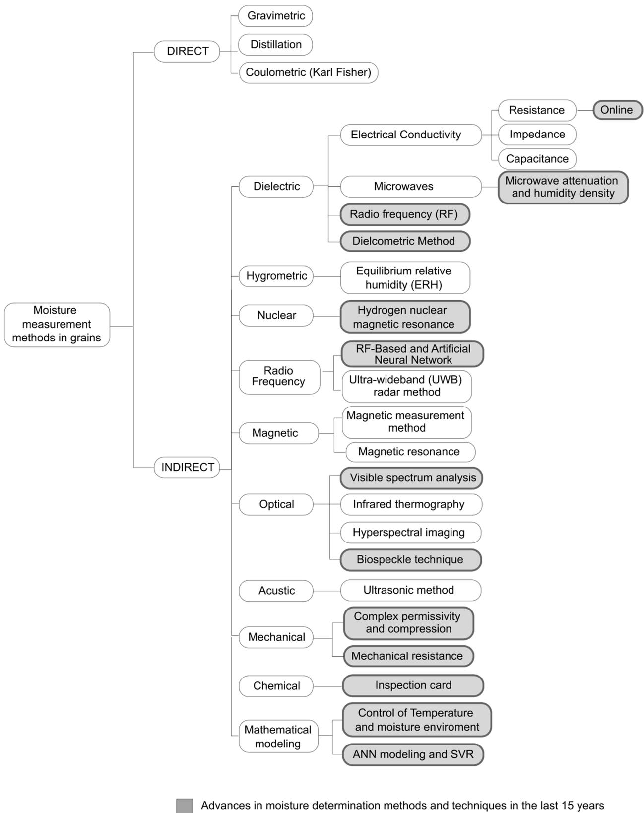
**Figure 2.** Classification of grain moisture measurement methods.
