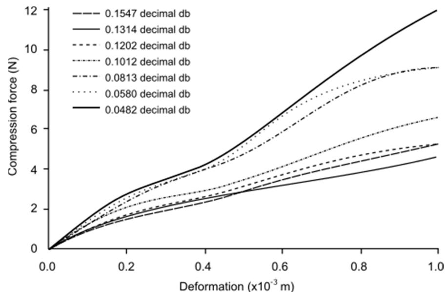
**Figure 22.** Strength as a function of deformation in *Crambe* (*Crambe abyssinica*) grains with different moisture contents.
