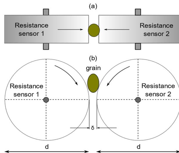
Figure 20. Structure of the single-grain moisture sensor: (a) top view; (b) front view.
