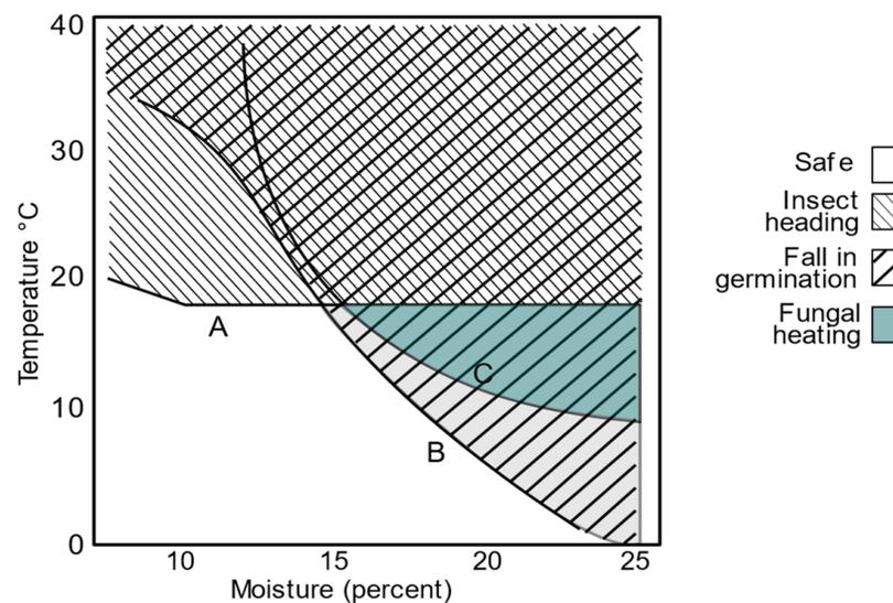
**Figure 1.** Effects in storage at different temperatures and moisture content.
