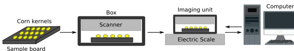
**Figure 17.** System operating procedure. 1–2, sampling; 3, imaging and weighing; 4, analyze.
