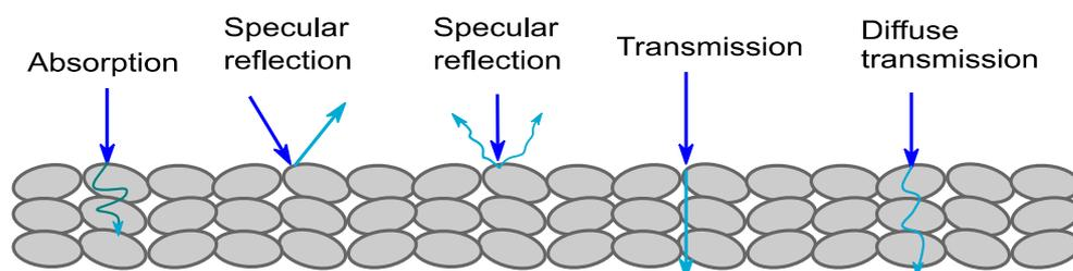
**Figure 14.** Interaction of light with solid bodies.
