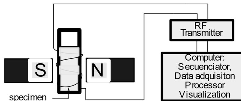
**Figure 9.** Schematic diagram of basic equipment for measuring RM.
