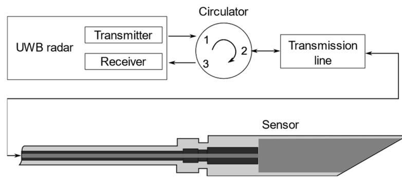
Figure 10. Schematic of portable UWB detection system.
