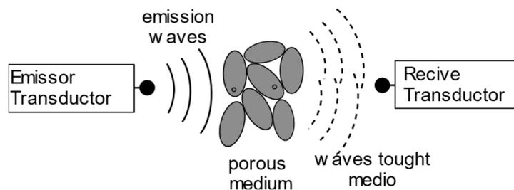
Figure 11. Schematic of the transducer arrangements facing each other within the method.
