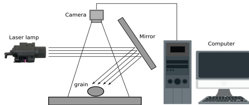
**Figure 21.** Schematic diagram of the biospeckle method of analysis.
