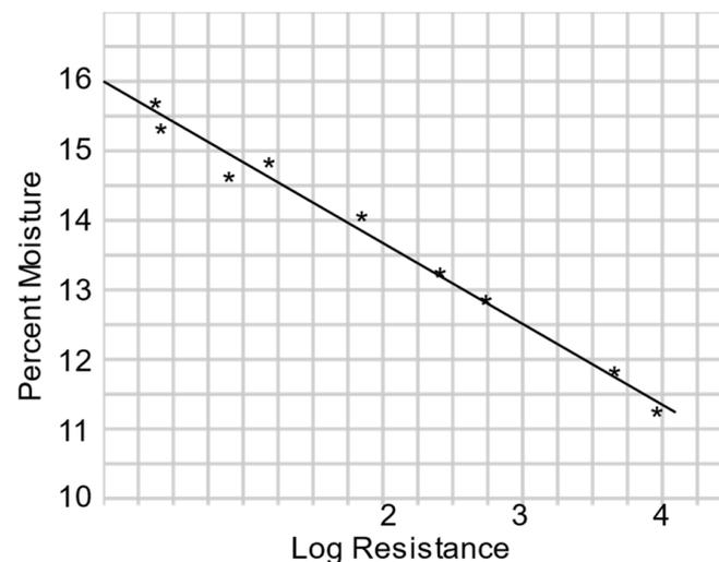
**Figure 4.** Relationship between moisture content and electrical resistance for wheat measured at 75 °F.
