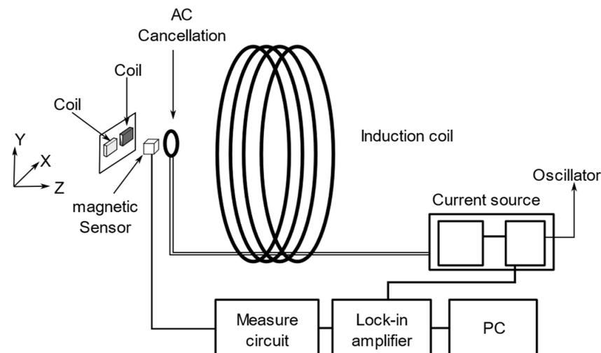
**Figure 7.** Schematic diagram of a magnetic measurement system that detects the moisture content of the grain.
