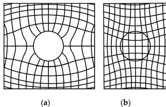
**Figure 24.** Representation of forces and equipotential lines of uniform electric field in a dielectric medium that passes through: (a) an unladen conductive sphere and (b) a dielectric sphere with a permittivity lower than that of the environment.
