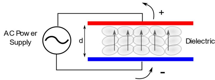
Figure 5. Grains in single plate capacitor.
