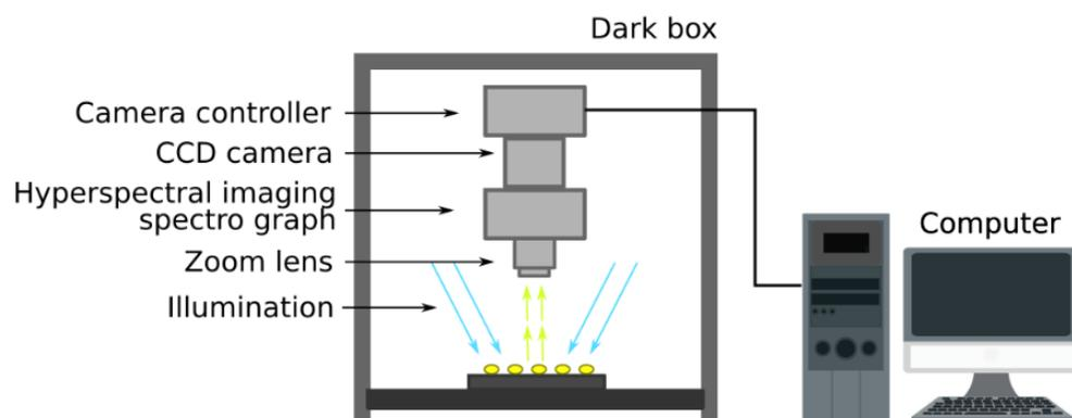
**Figure 15.** Schematic of the hyperspectral reflectance imaging system.
