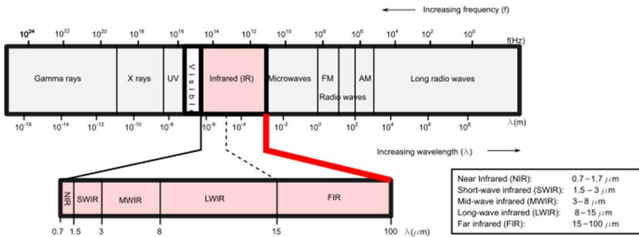
**Figure 12.** The electromagnetic (EM) spectrum. As evidence, the infrared (IR) region in which the reflected IR (0.7–3.0  $\mu\text{m}$ ) and emitted IR (3.0–100  $\mu\text{m}$ ) are more detailed.
