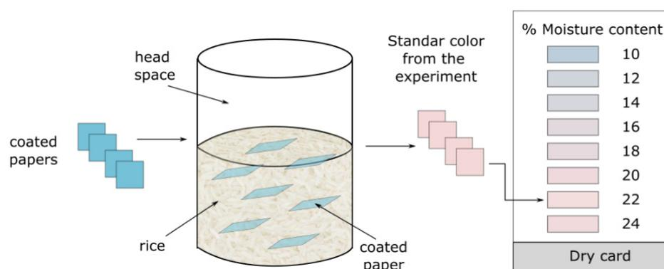
Figure 23. Moisture inspection card.
