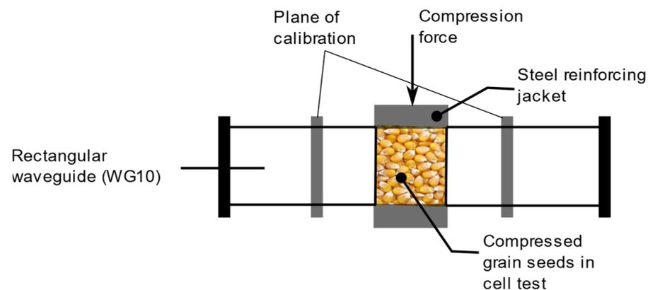
**Figure 19.** Waveguide cell setup for the compressed grain bulk sample.
