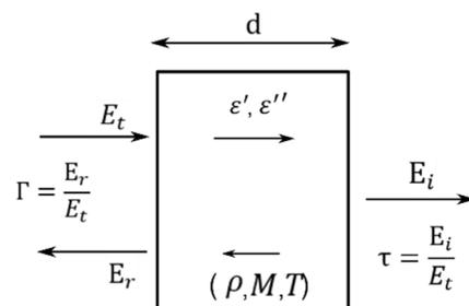
Figure 6. Diagram of wave-dielectric material interaction.
