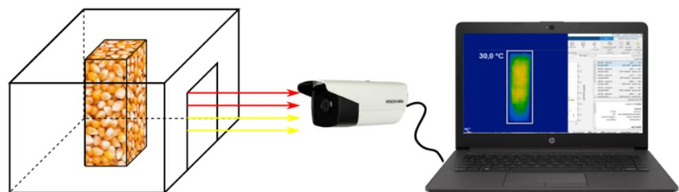
**Figure 13.** System employed to capture the thermographic images of grain samples.
