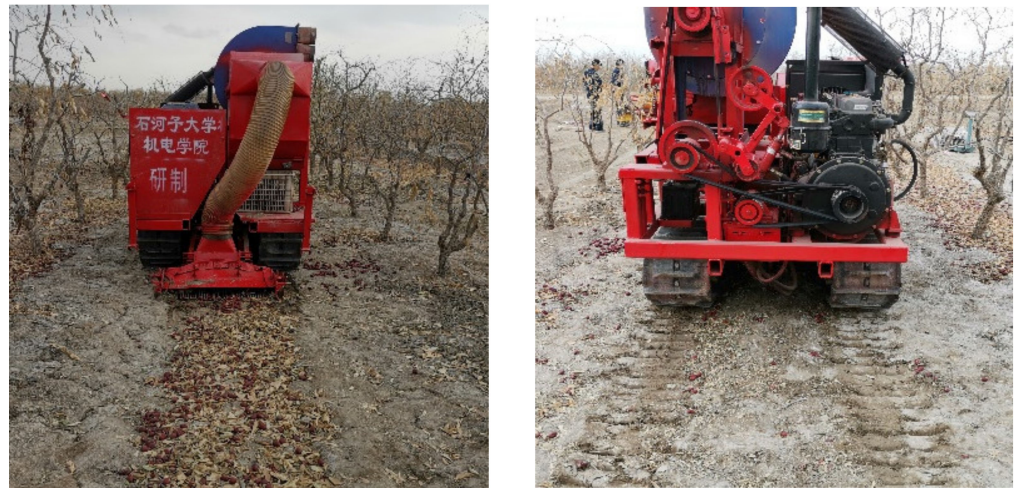
Figure 10. Field verification test process and work performance of the provoke-suction type harvester for ground jujube fruit (PSH). The Chinese in left image means “developed by the College of Mechanical and Electrical Engineering, Shihezi University”.
