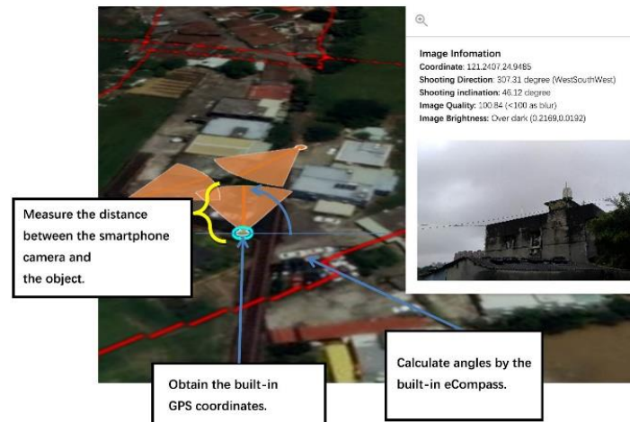
Figure 3. The crucial technique for the agricultural survey APP is to measure the distance between the camera and the object.
