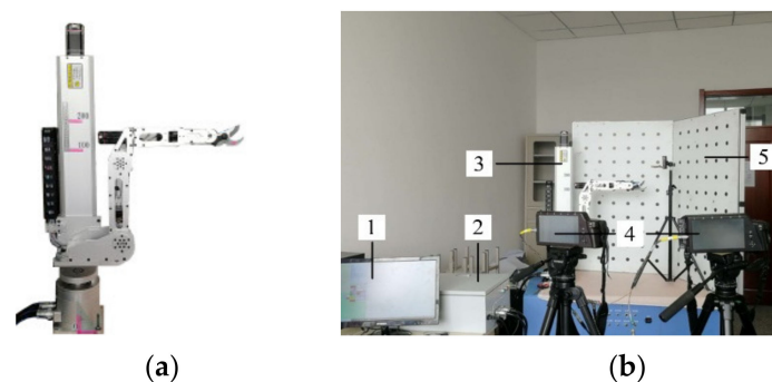
Figure 11. The platform for the manipulator performance test. (a) Prototype and (b) test platform. 1. PC machine; 2. Control box; 3. Manipulator; 4. 3D high-speed camera; and 5. Calibration plate.
