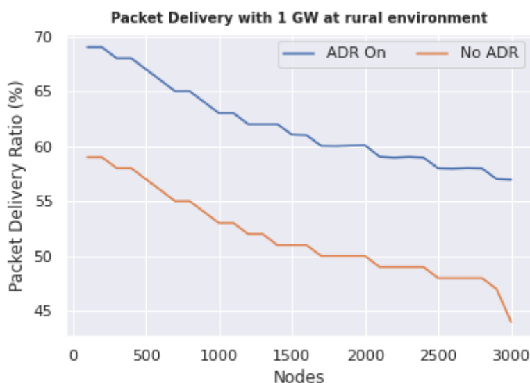
Figure 11. Packet delivery ratio to the network server with a single gateway under propagation conditions simulating a rural environment.
