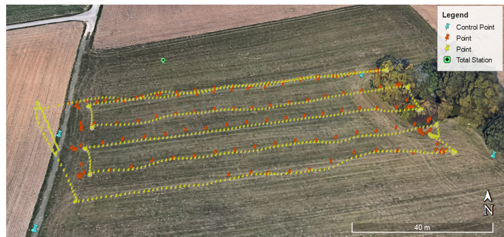
Figure 4. Satellite view with the positions of the prism (yellow pins) and the positions of the images (red pins). The direction of movement was as close as possible along the East–West axis (E–W). The TS and the four control points that were used for the stationing are also indicated (Landsat / Copernicus, Google Earth, edited).
