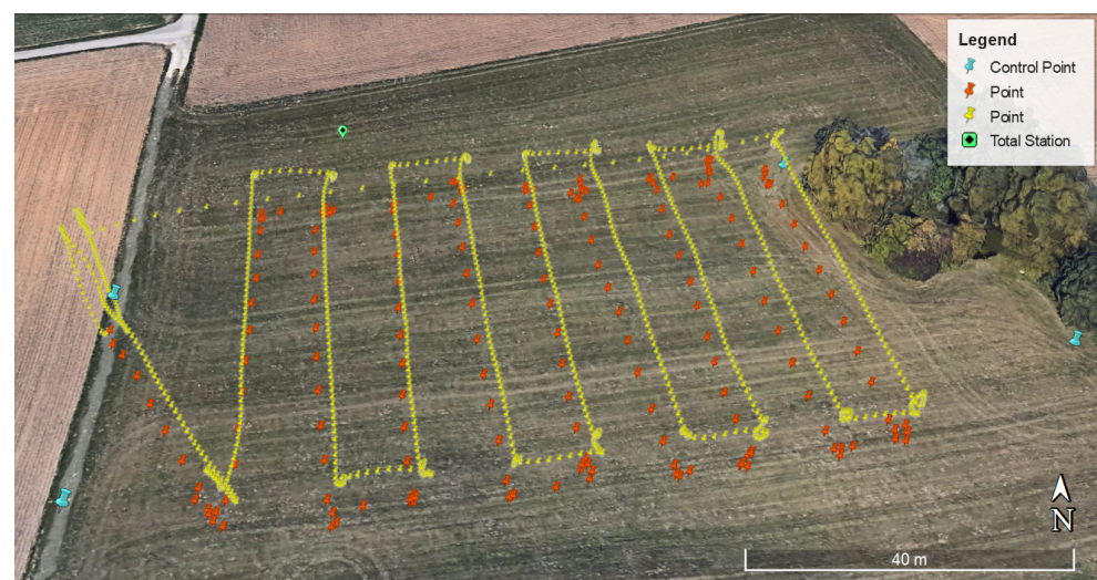
Figure 5. Satellite view with the positions of the prism (yellow pins) and the positions of the images (red pins). The direction of movement was as close as possible along the South–North axis (S–N). The TS and the four control points that were used for the stationing are also indicated (Landsat/Copernicus, Google Earth, edited).
