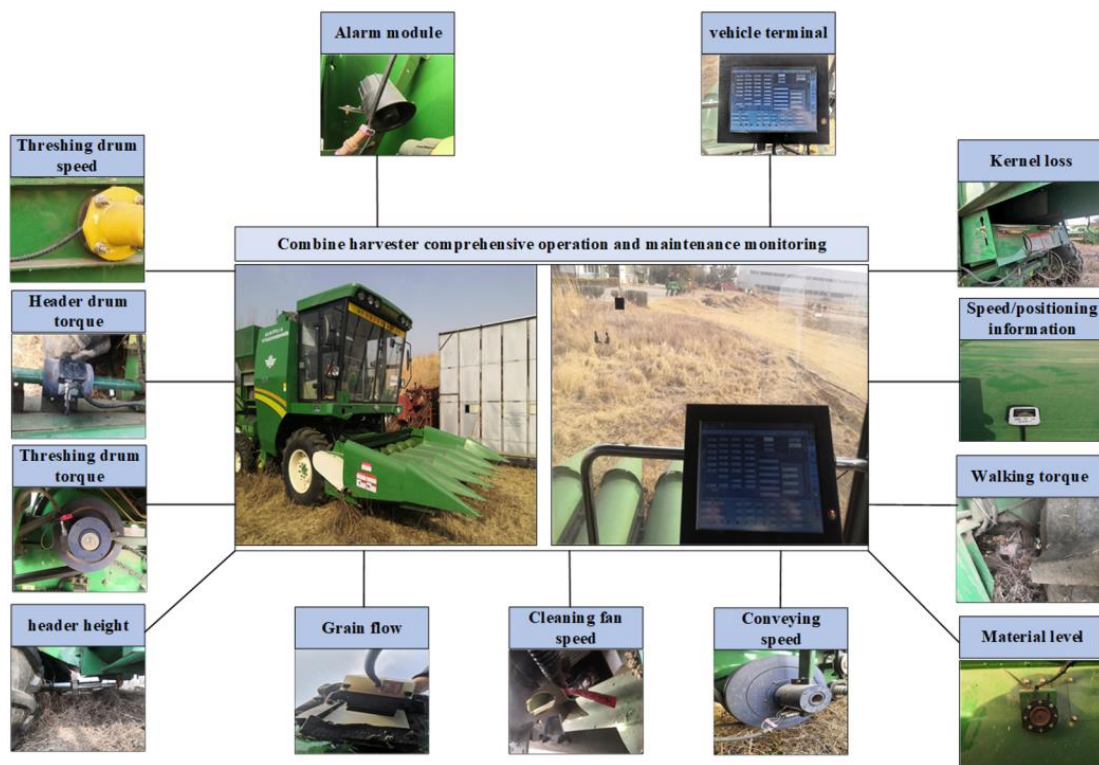
Figure 1. Structure of fault diagnosis and monitoring system of combine harvester.
