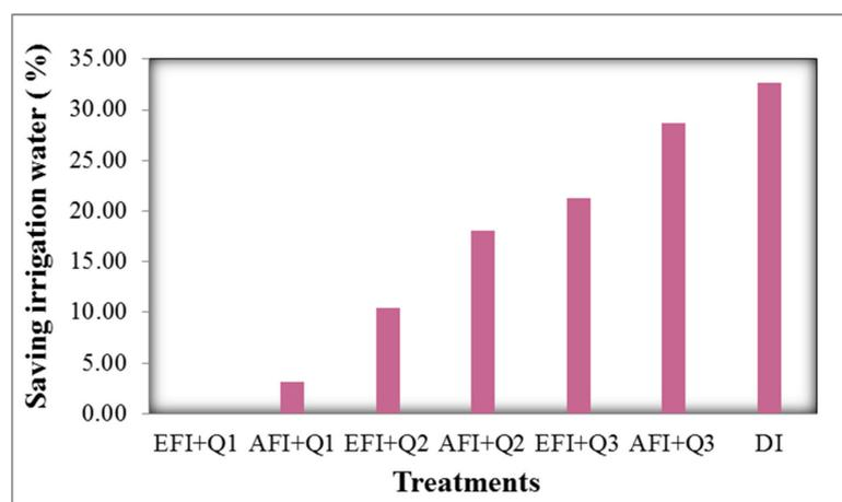
**Figure 6.** Effect of irrigation method (EF, AF, and DI) and flow rate (0.47 (Q1), 0.95 (Q2), and 1.43 L/s (Q3)) on irrigation-water-saving percentage across two years.
