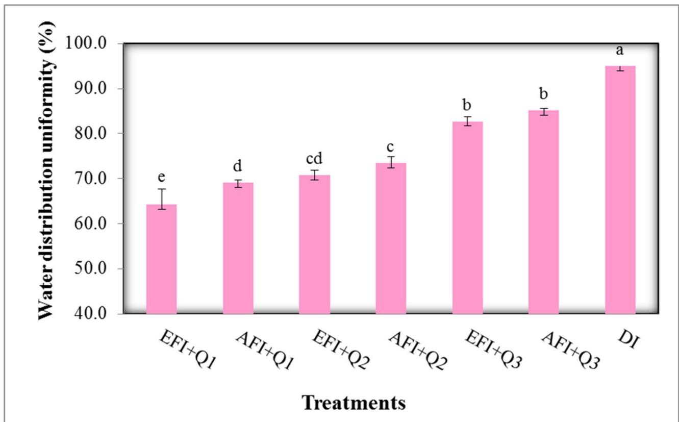
**Figure 2.** The effect of irrigation systems (EFI, AFI, and DI) and flow rates (0.47 (Q1), 0.95 (Q2), and 1.43 L/s (Q3)) on the water distribution uniformity across two seasons. Mean values followed by the same letter were not significantly different at the 5% level between treatments.
