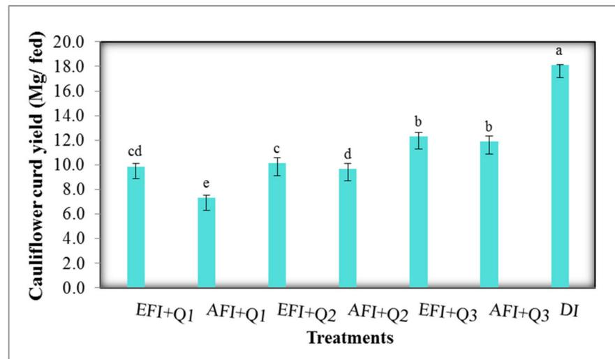
**Figure 4.** Effect of irrigation method (EFI, AFI, and DI) and flow rate (0.47 (Q1), 0.95 (Q2), and 1.43 L/s (Q3)) on cauliflower curd yield across two seasons. Mean values followed by the same letter were not significantly different at the 5% level between treatments.
