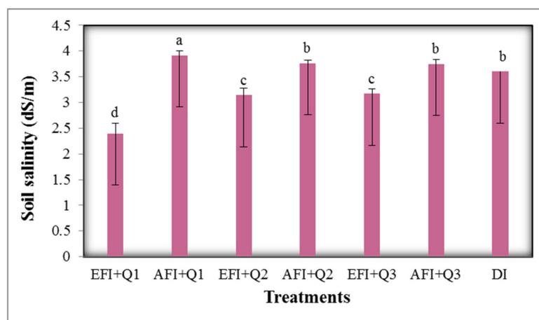
**Figure 7.** Effect of irrigation method (EF, AF, and DI) and flow rate (0.47 (Q1), 0.95 (Q2), and 1.43 L/s (Q3)) on soil salinity after cauliflower harvesting across the two years. Mean values followed by the same letter were not significantly different at the 5% level between treatments.
