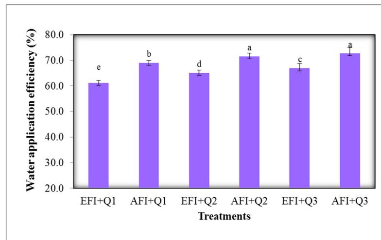
**Figure 3.** Effect of irrigation systems (EF and AF) and flow rates (0.47 (Q1), 0.95 (Q2), and 1.43 L/s (Q3)) on water application efficiency across the two seasons. Mean values followed by the same letter were not significantly different at the 5% level between treatments.
