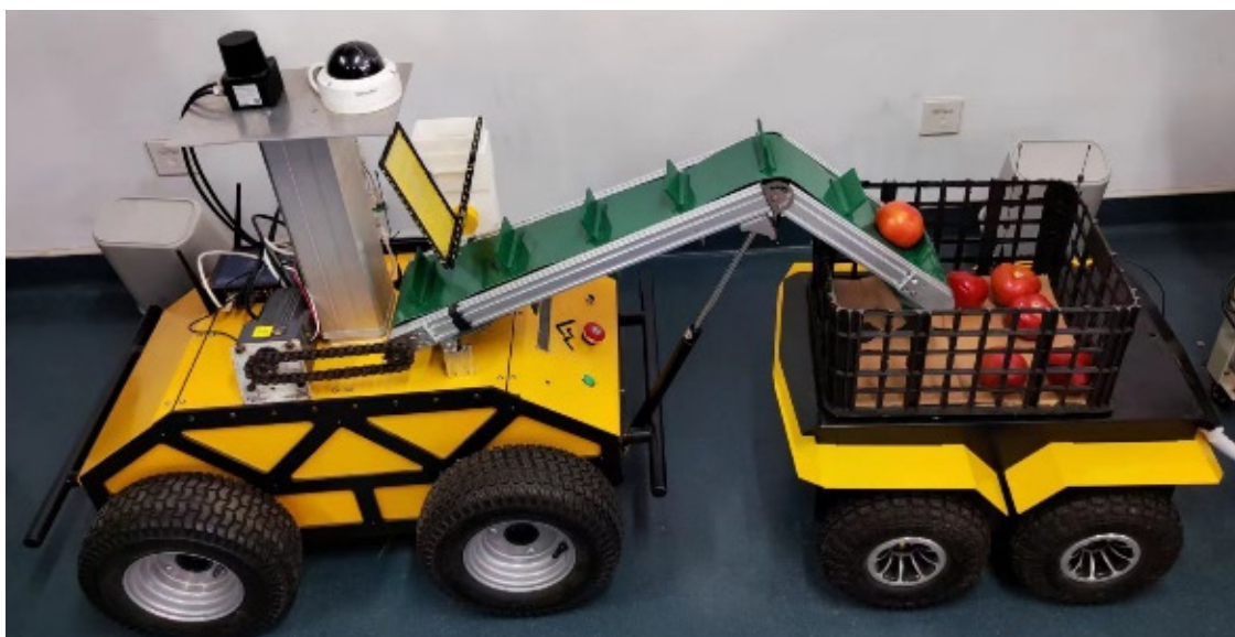
Figure 13. Prototype test of post-harvest collection device.
