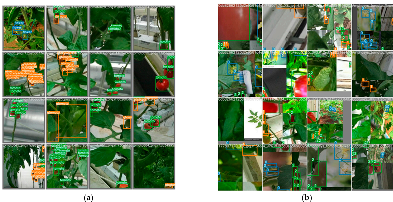
Figure 6. The data set representation, (a) Ground Truth Training Data, (b) Ground Truth Augmented training data. For augmented data, 0, 1, and 2 labels represent flower, green tomato, and red tomato classes, respectively.
