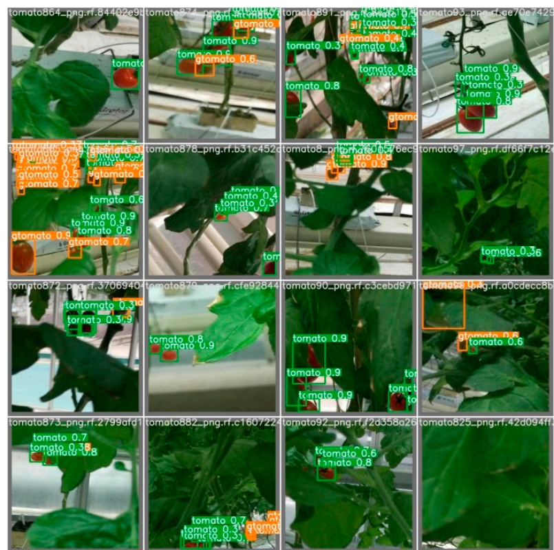
Figure 11. Obtained test results batch with accuracy for Tomato detection model. Here, green and orange colored bounding boxes represent red tomato and green tomato classes, respectively.
