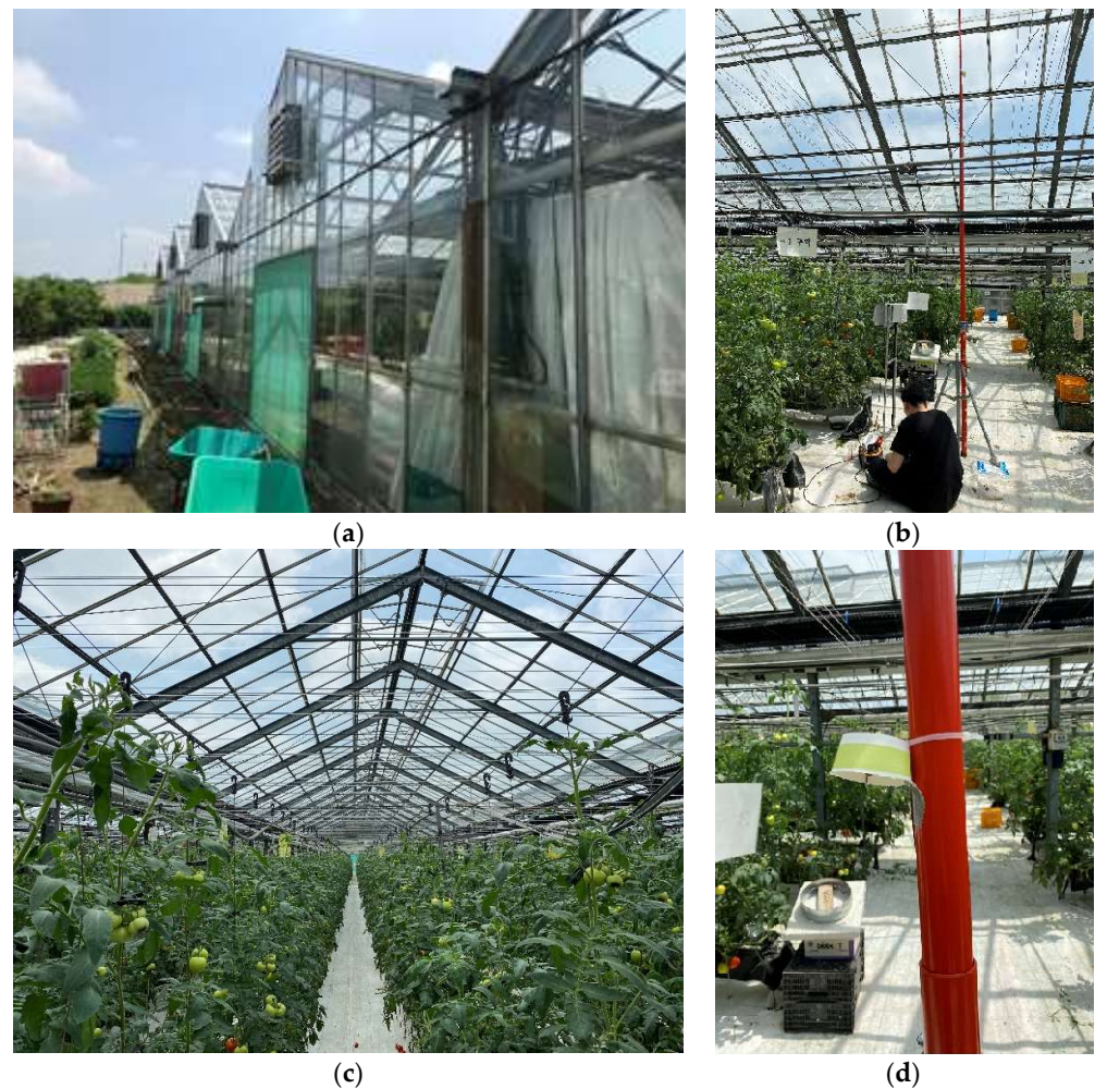
Figure 4. Experimental greenhouse located in Moga-myeon, Icheon-si, Gyeonggi-do Province ( 37^{\circ}18'N , 127^{\circ}48'E ) and field experiment (a) External view of the experimental greenhouse, (b) Sensor installation for measuring vertical air temperature, (c) Internal view of the experimental greenhouse and (d) Sensor installation to avoid direct radiation.
