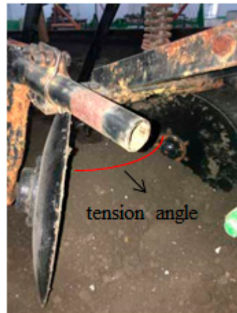
Figure 6. Double-disc-type eight-character cover.
