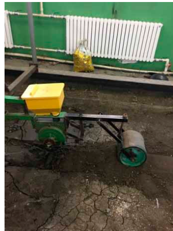
Figure 7. Cylindrical compacting roller.
