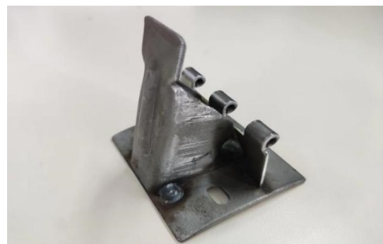
Figure 20. Welding forming of duckbill parts.
