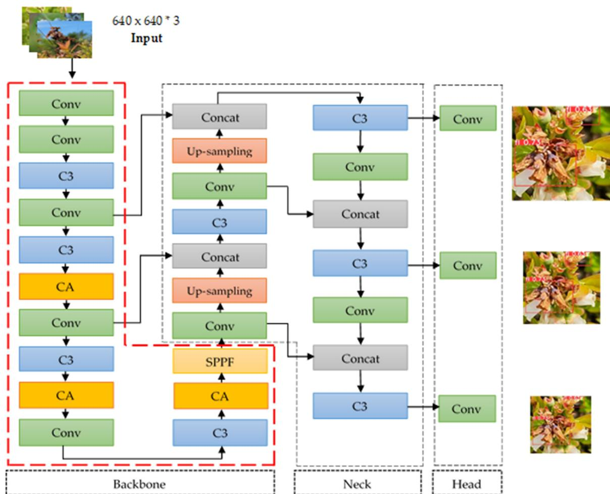
**Figure 4.** The improved Yolov5s-CA network model structure.
