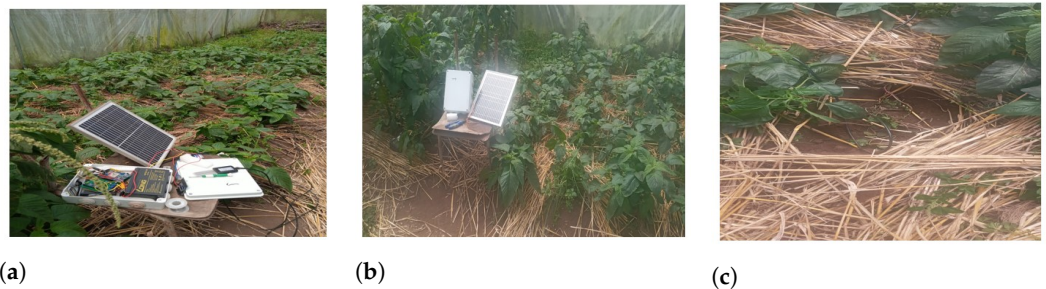
Figure 11. Visual depiction of IoT sensor setup; (a) sensors, battery and solar; (b) sensor assembled; (c) sensor deployed in cropland.
