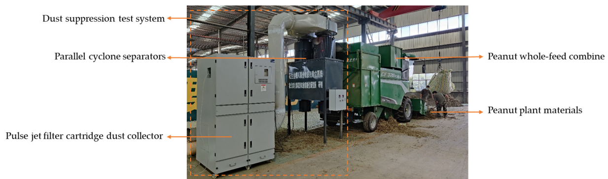
Figure 5. Experiment of the dust suppression test system.
