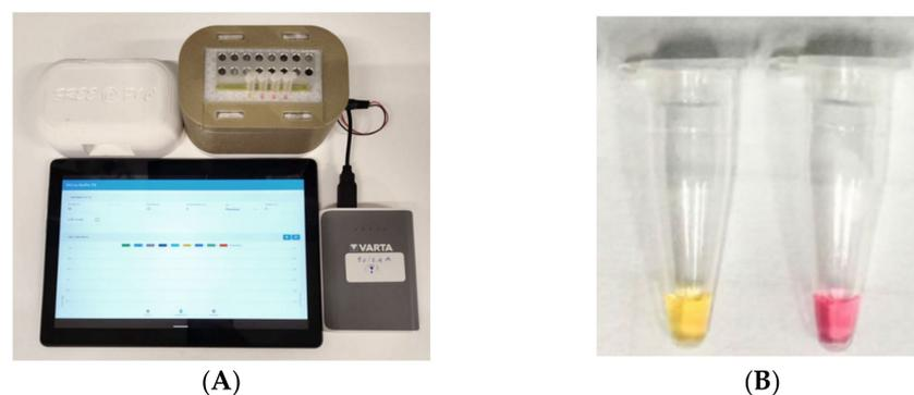
**Figure 1.** (A) Overview of the 3D-printed portable thermal block device. The plastic box contains a heating metal block, set to operate at 65 °C for 30 min. The device is powered by a portable power bank and connected via Bluetooth to a tablet. (B) The positive reaction (amplified DNA) is visualized by the color change from pink (negative signal) to yellow (positive signal).
