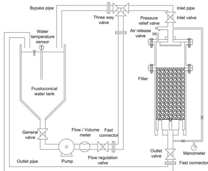
**Figure 2.** Experimental laboratory setup.
