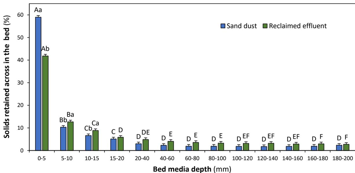
**Figure 5.** Average ( $\pm$  standard error) of the percentage of solids retained across the whole media bed in each slice of bed regarding the type of particles added. Different small letters show significant differences ( $p < 0.05$ ) between sand dust and reclaimed effluent for a given bed slice. Different capital letters mean significant differences ( $p < 0.05$ ) between bed slices for a given type of particle added.
