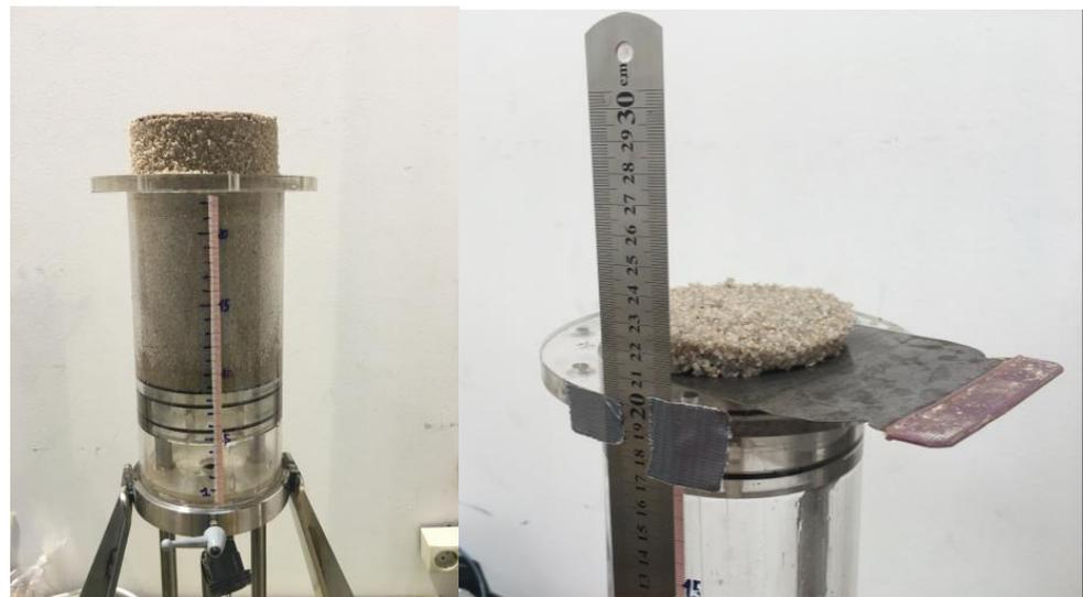
**Figure 3.** Extraction of bed slices in the experimental filter.
