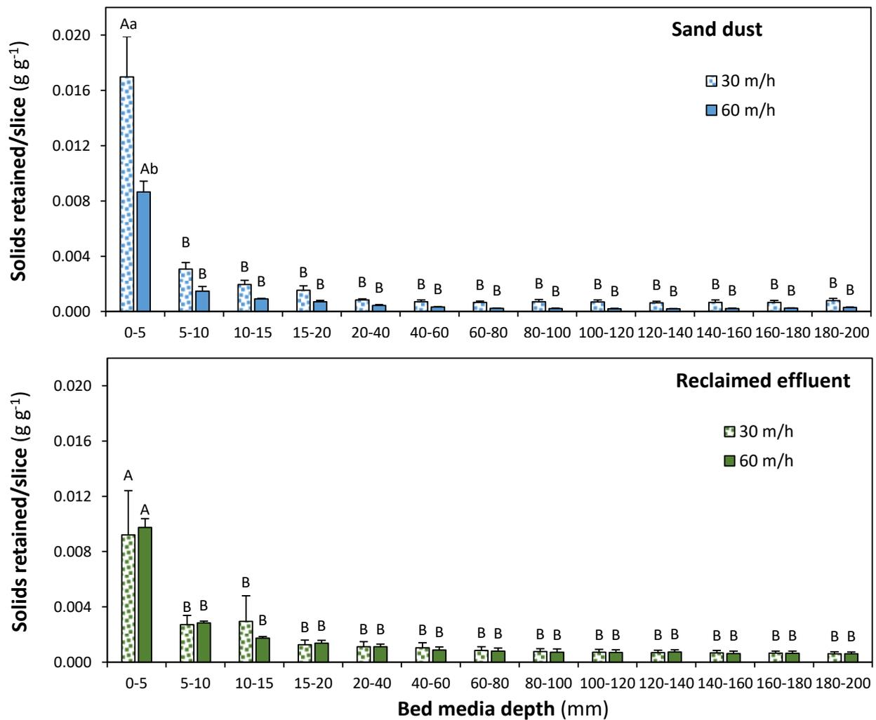
**Figure 4.** Average ( $\pm$ standard error) of the total suspended solids (g) retained per mass (g) of slice bed across the whole media bed depth regarding the type of particles added and the target filtration velocity. Different small letters show significant differences ( $p < 0.05$ ) between filtration velocities for a given bed depth. Different capital letters show significant differences ( $p < 0.05$ ) between media bed depths for a given filtration velocity.
