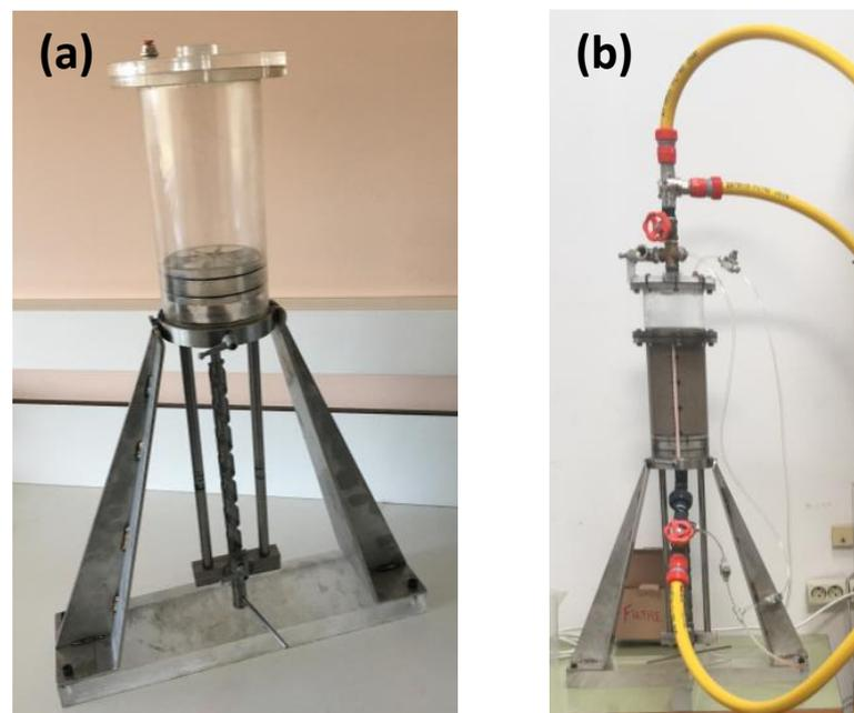
**Figure 1.** (a) Experimental filter built for the experiment before and (b) after the insertion of the sand bed and the necessary fittings for conducting the experiment.
