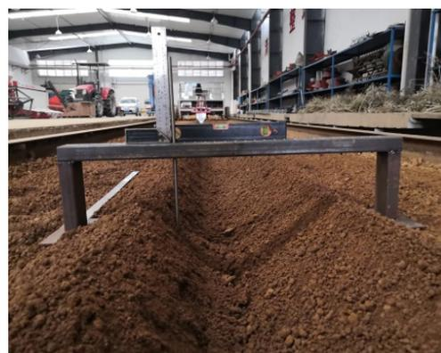
**Figure 3.** Furrow contour measuring device.
