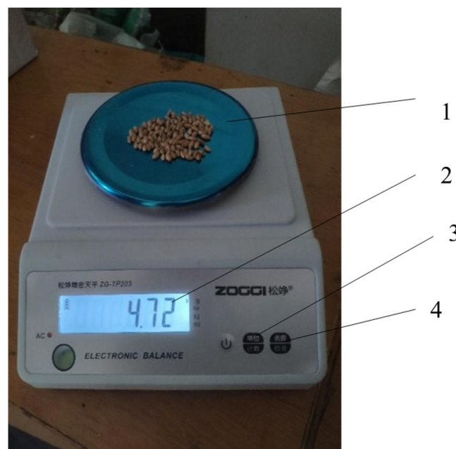
Figure 6. Thousand seed weight measurement by the 100-seeds method. 1. Wheat seed. 2. Display interface. 3. Counting unit. 4. Scaling unit.
