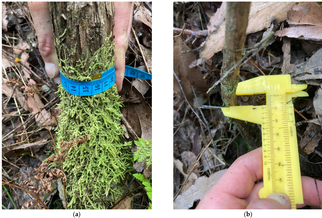
Figure 3. A measuring tape was used to measure the circumference of stems >25 mm in diameter (a). A caliper was used to measure the diameter of stems <25 mm in diameter (b). The measurements are taken 100 mm above the ground.
