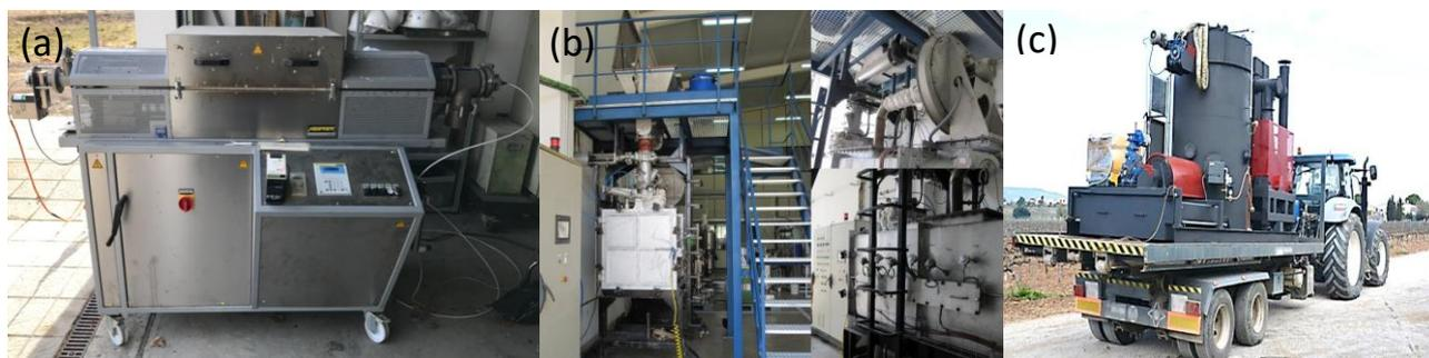
**Figure 1.** Photograph of the (a) semi-pilot reactor, (b) pilot reactor and (c) industrial reactor.
