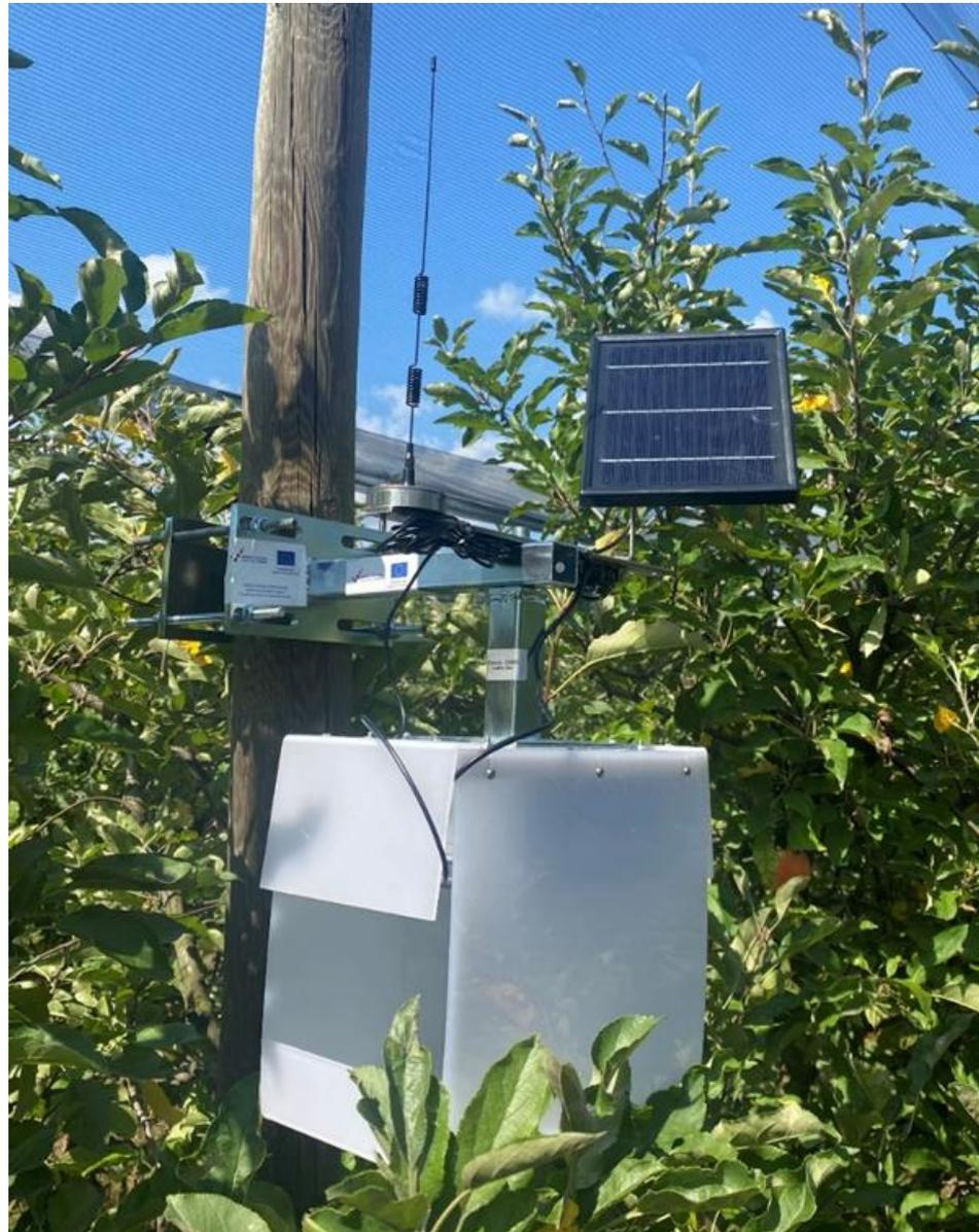
**Figure 1.** The smart trap prototype installed in the orchard.
