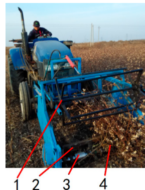
Figure 13. Field test photo: 1. Reel wheel 2. V-shaped tooth roller 3. Torque transducer 4. Cotton stalks.
