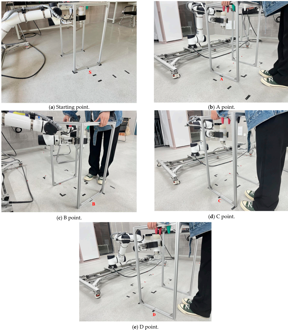
Figure 17. Dynamic response of the robot cup test diagram: (a–e) the movement of the model from the origin to point D and the following real-time process of the robot arm.
