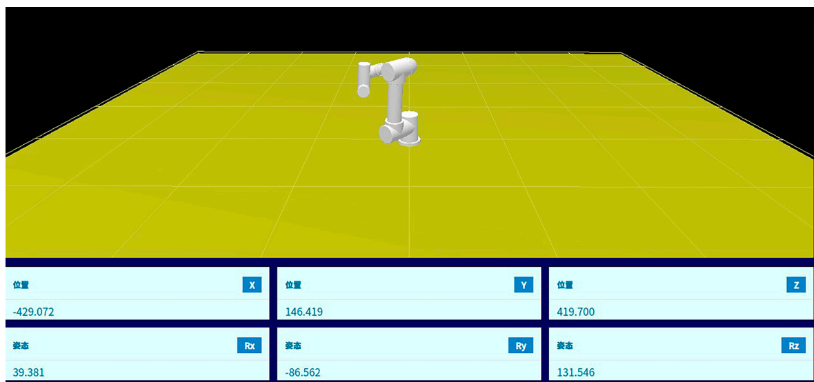
Figure 15. Actual coordinate diagram in the software interface. The term "位置" refers to displacement, while "姿态" denotes angle.
