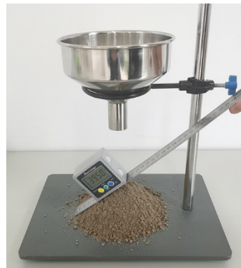
Figure 2. Stacking angle determination of soil.
