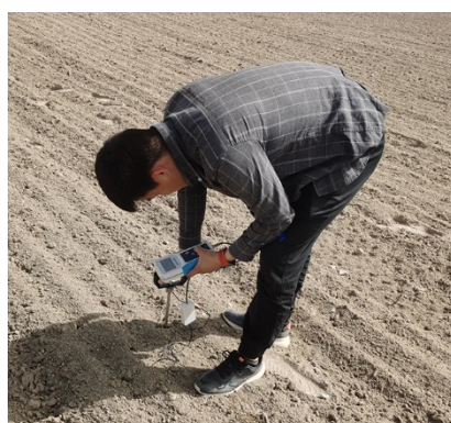
Figure 1. Firmness determination of soil.
