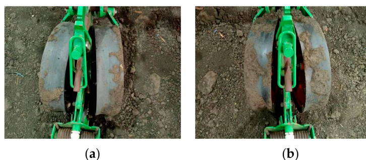
Figure 7. Planting unit with different gauge wheels: (a) profiling gauge wheel with irregular cavity; (b) profiling gauge wheel with symmetrical cavity.
