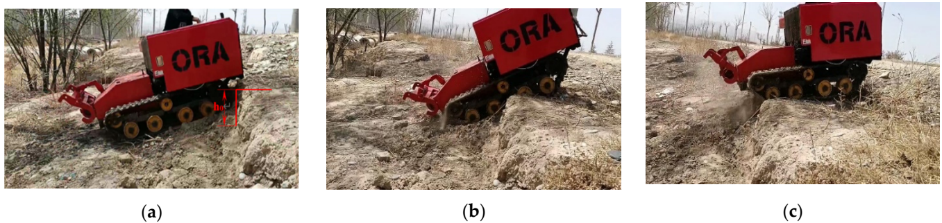
Figure 19. Obstacle-passing test: (a) before crossing the barrier; (b) obstacle crossing; (c) after crossing the obstacle.
