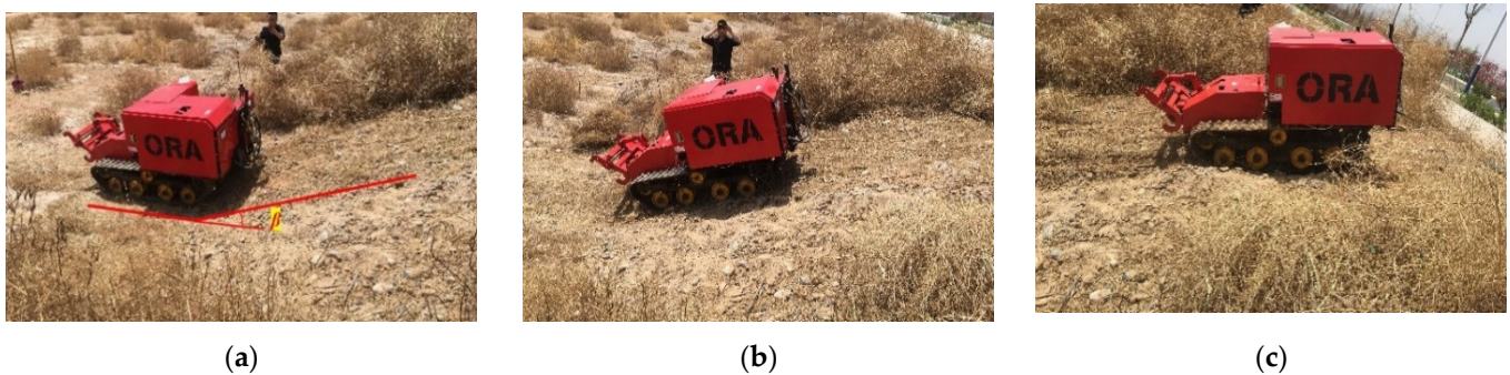
Figure 18. Hill-climbing performance test: (a) the beginning of the climb; (b) climbing stage; (c) late climbing stage.
