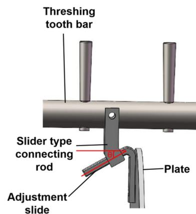
Figure 3. Diagram of adjusting the angle of the slide rail.
