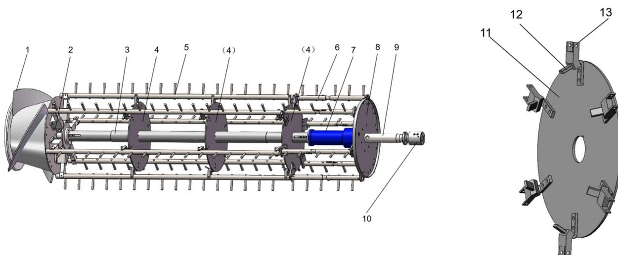
Figure 1. Schematic diagram of the structure of the variable-diameter threshing drum with movable radial plates: 1. feeding wheel, 2. side width plate adjustment mechanism, 3. sleeve, 4. support width plate mobile type adjustment mechanism, 5. fixed gear rod, 6. telescopic gear rod, 7. single piston rod hollow hydraulic cylinder, 8. rear side width plate, 9. spindle, 10. hydraulic rotary joint, 11. width plate, 12. adjustment slide, 13. slider type linkage.
