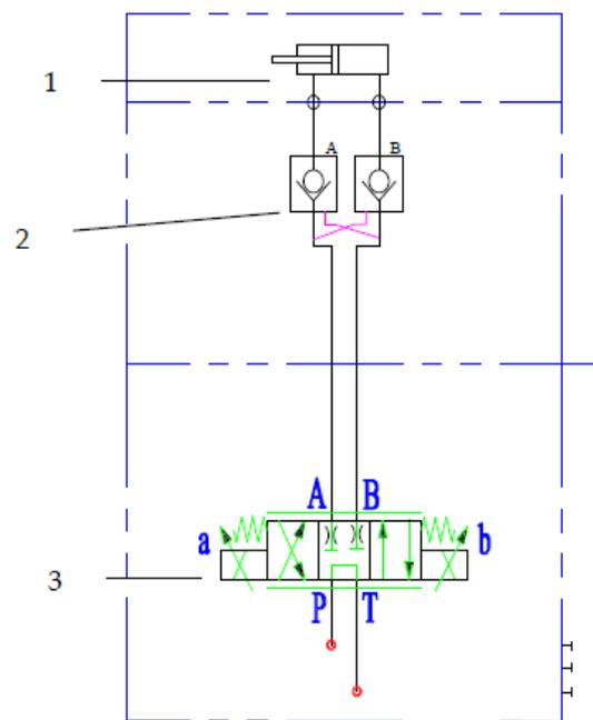
**Figure 2. Hydraulic system schematic:** 1. hollow hydraulic cylinder, 2. hydraulic lock, 3. three-way four-way solenoid proportional reversing valve.
