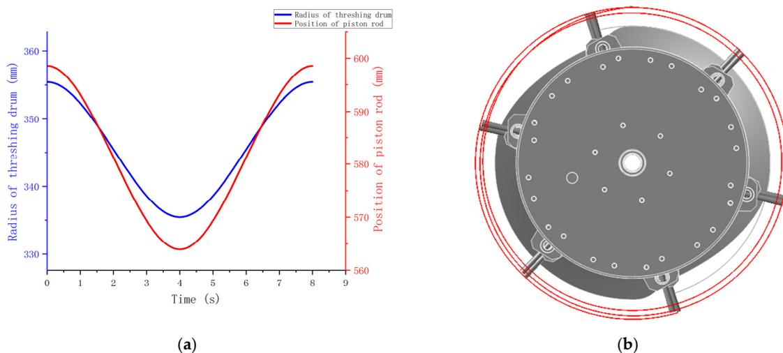
**Figure 7. Simulation of diameter adjustment of RecurDyn-based variable-diameter threshing drum with movable radial plates. (a)** Piston rod position along the main shaft and drum diameter variation diagram; **(b)** Marker 6 motion track.
