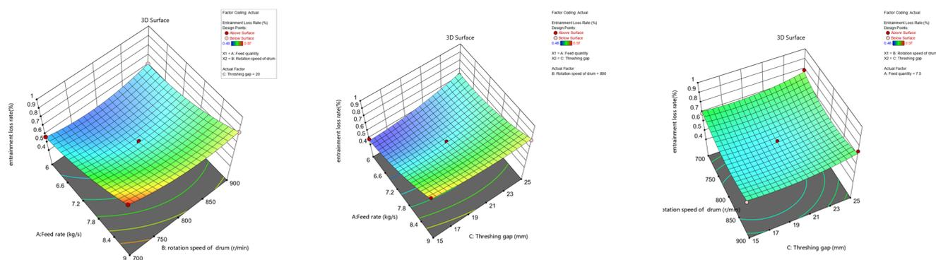
Figure 9. Response surface of each factor on entrainment loss rate.
