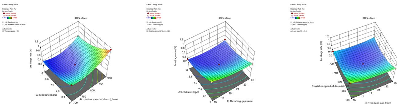
Figure 11. Response surface of each factor on breakage rate.
