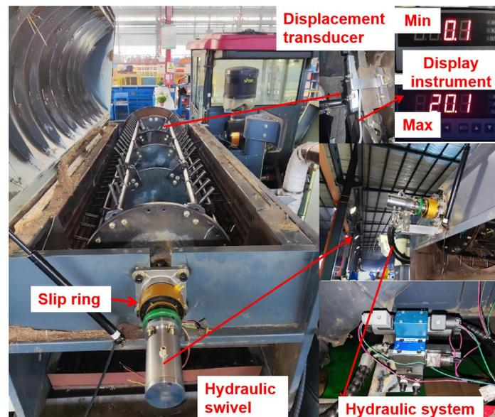
**Figure 8.** Variable-diameter threshing drum with movable radial plates and hydraulic system and related accessories.
