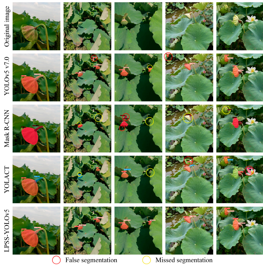
Figure 15. Segmentation effects of different instance segmentation models on the sample test images.
