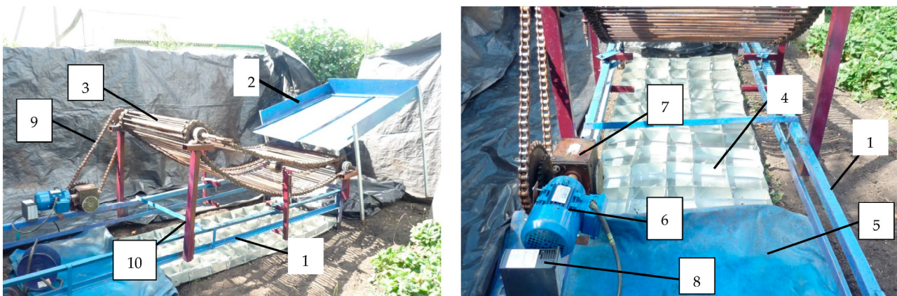
Figure 2. Laboratory setup for studying the tribological properties of an elastoplastic material when interacting with an absolutely solid body: 1—frame; 2—container for preliminary placement of a heap; 3—separating rod elevator; 4—a tray for collecting impurities; 5—tarpaulin of separated products; 6—electric motor; 7—single-stage gearbox; 8—frequency converter; 9—chain transmission; 10—support racks.
