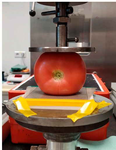
Figure 5. Compression test integrated with surface pressure measurement.
