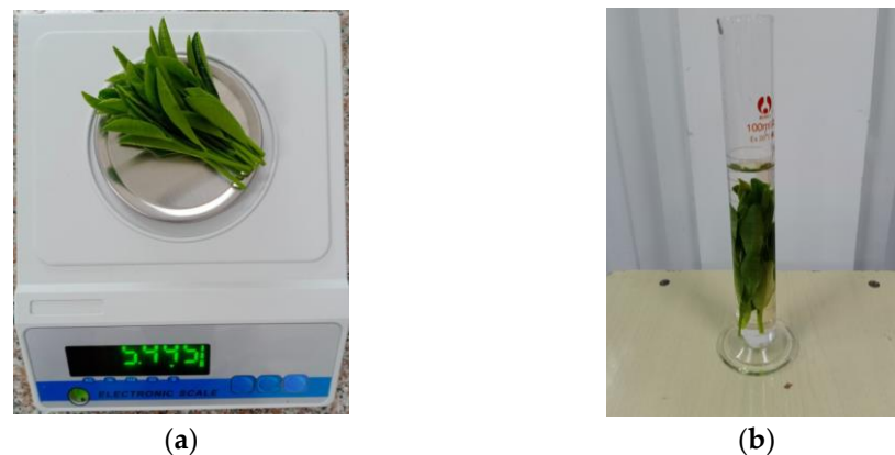
Figure 2. Density measurement of fresh tea leaves: (a) quality measurement of tea leaves; (b) volume measurement of tea leaves.
