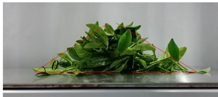
Figure 4. Physical repose angle test of fresh tea leaves.
