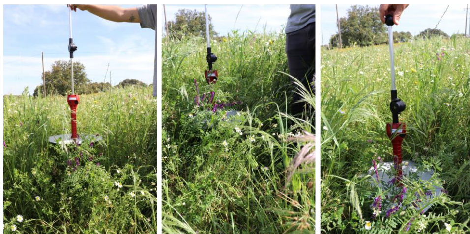
Figure 15. Measurements with the rising plate meter (RPM) in the field of the grassland mixture for cutting in the validation phase.
