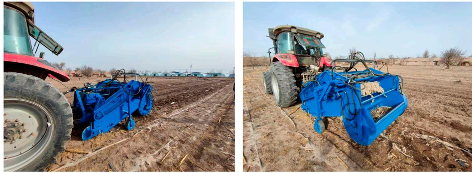
**Figure 14.** Field test of operation performance of residual film-recycling machine.
