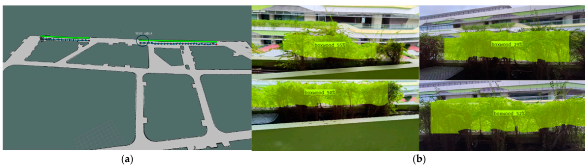
Figure 13. (a) Deployment zone for testing the pruning algorithm; (b) detection of pruning subjects using YOLOv8.
