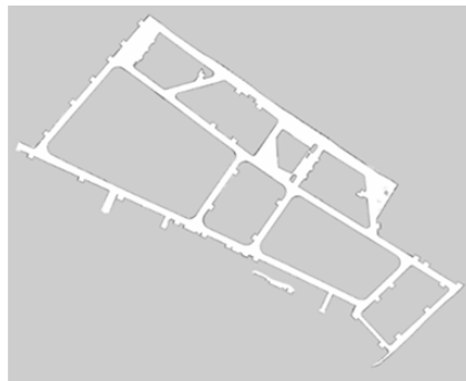
Figure 6. A 2D map of the deployment zone retrieved from the 2D LiDARs and IMUs.
