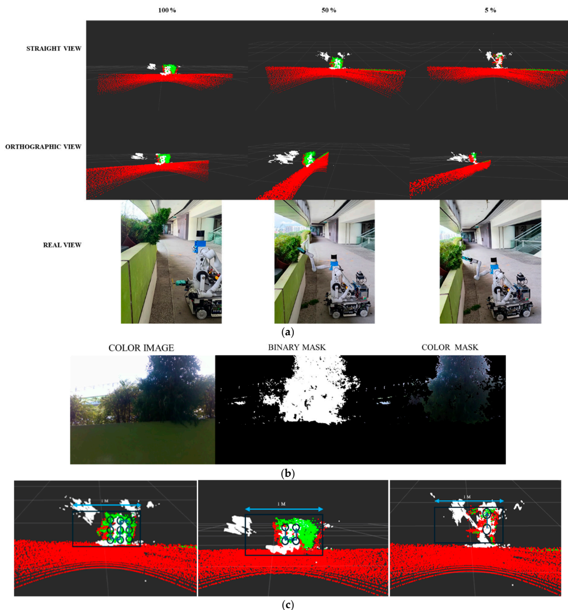
Figure 14. (a) Detection of target points at various stages of pruning operation; (b) original color image, binary mask, and color mask of the target zone; (c) waypoint estimation at various stages of pruning.
