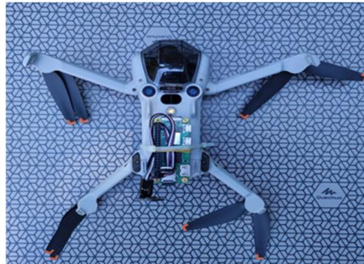
**Figure 1.** Equipping the DJI Mini 4 Pro drone (Dà-Jiāng Innovations, Shenzhen, Guangdong, China) with the Vishay VEML 6075 digital sensor.
