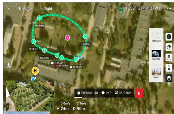
**Figure 2.** Route planning through waypoints (screenshot): the green circles represent intermediate points, numbered from 1 to 7, while the pink diamond located at the center of the flight path represents the point of interest (POI), noted with 1.
