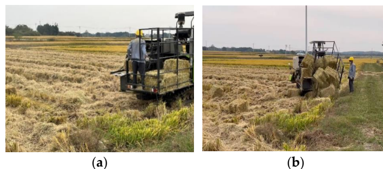
Figure 3. Straw harvesting process of the pickup baler. (a) Manual bale stacking; (b) bale unloading at the field edge.
