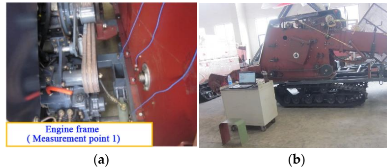
Figure 9. Vibration test testing scenarios. (a) Engine position measurement point arrangement; (b) indoor vibration testing.
