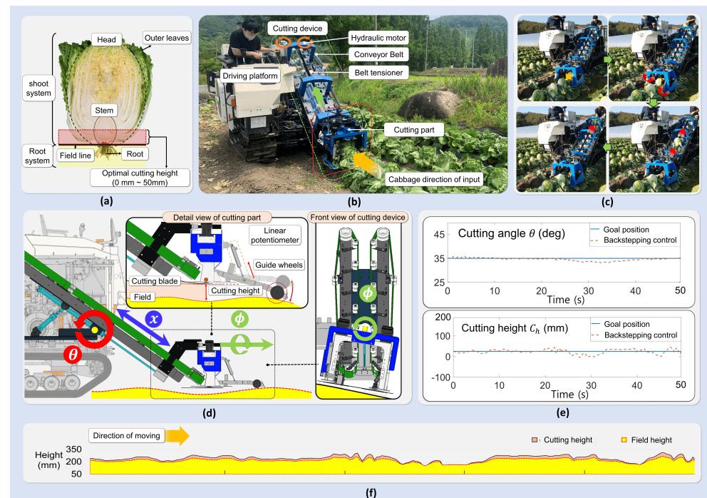
Figure 5. Korean cabbage harvester [27]; (a) structure of a Korean cabbage, (b) harvesting process of the developed harvester, (c) attitude control system of the cutting device, (d) verification of goal position following, and (e,f) harvesting of Korean cabbage using an attitude control system.
