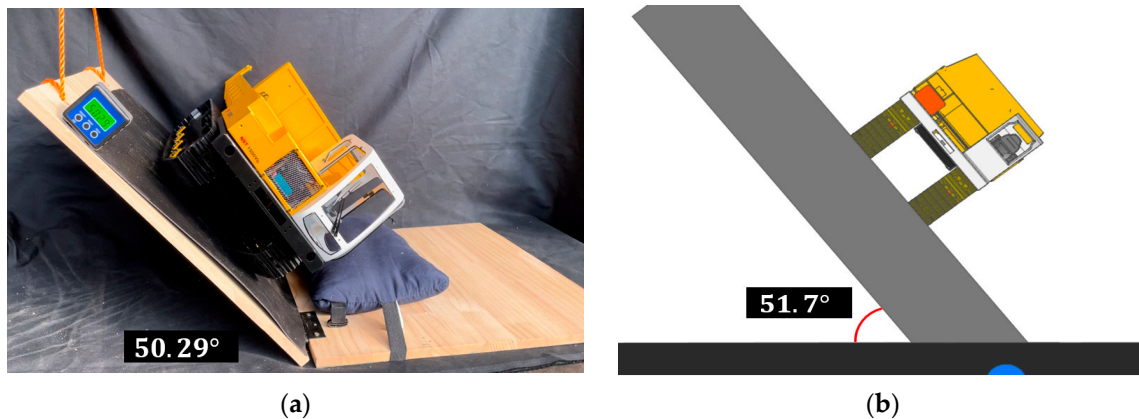
Figure 14. Practical test and simulation of static sidelong falling angle test: (a) practical test; (b) simulation.
