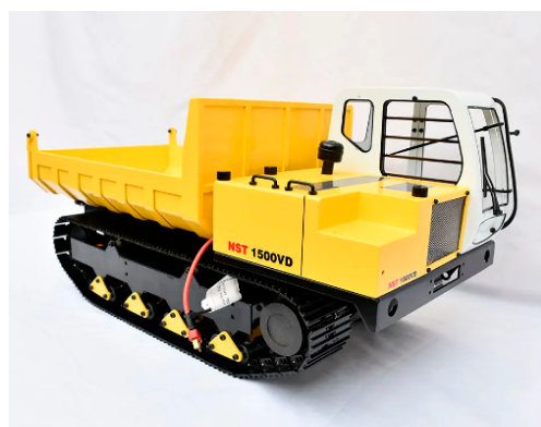
Figure 4. Photograph of miniature tracked forestry tractor.
