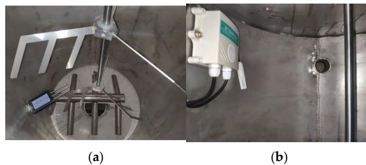
**Figure 13.** Installation position of each sensor. (a) Installation location of soil temperature–humidity sensor; (b) installation location of air temperature–humidity–oxygen concentration sensor.
