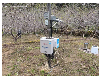
Figure 7. The orchard meteorological station collects environmental data within the orchard and promptly uploads the data to a cloud platform for storage.
