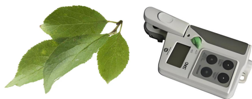
Figure 6. Leaves and the SPAD-502 chlorophyll analyzer: the SPAD-502 instrument is used to clamp the leaves and obtain chlorophyll values.
