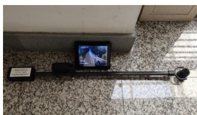
Figure 5. The leaf area index (LAI) measuring instrument, with its fish-eye lens facing upwards, is placed horizontally above the crown of the tree during measurement.
