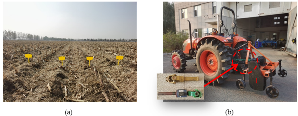
Figure 9. (a) Field experiment site and (b) experimental equipment: I: torque sensor.
